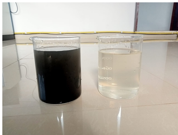
Left: Inlet from MPS | Right: Effluent Water
